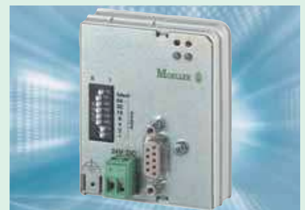
Fieldbus connection DE4-NET-DP2 for direct connection to PROFIBUS DP (DIN 19245 part 1 and 3)
