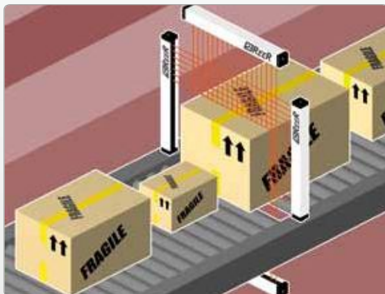
Two-dimensional detection of objects in transit on conveyor systems with use of 2 light curtains. If necessary, the calculation of the volume can be made by means of a third horizontal light curtain, or considering the transit speed
