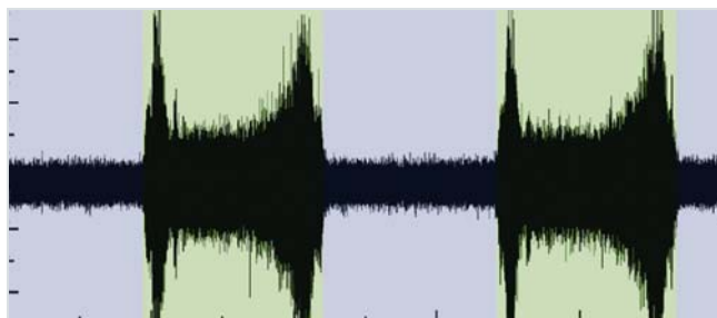
Signal from structure-borne sound sensor with defective valve
